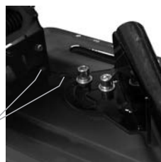
Positioning holes of the base for angled cuts.
