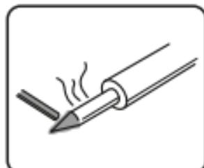
The soldering tips are chrome galvanized on the surface and should be bright silver without waste or welding on it.
