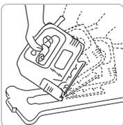
Pressure in the shoe lips with the blade exactly on lined **NOT MOVE THE SAW FORWARD ALONG ITS CUT** until the saw blade has completely entered the material and the shoe comes to rest flat on its surface.
