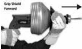
2. Slide the grip shield back to grip cable. Then gently squeeze the trigger and move the machine toward the drain opening. **DO NOT FORCE THE CABLE.** The job won't go any faster and you could kink the cable.
