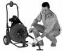
6. Select the proper cutting tool. A good tool to start with is the Spearhead or 2" U Cutter. If you are having difficulty getting around a P-Trap or close bend, try the flexible leader. After the line has been opened, follow with larger blades, which scrape the inside edges of the pipe, assuring a real cleaning job.
