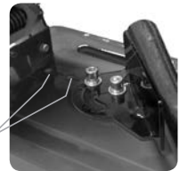
Positioning holes of the base for angled cuts.
