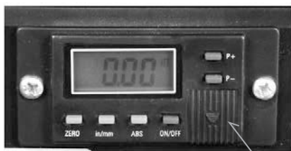
Compartment for the batteries (2 of 1,2 V)
